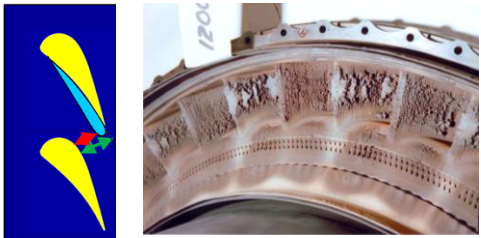
T4 vs NGV Accumulation Factor After 7 mins Exposure to Blend#2 or Black Scoria (concentrations in the legend are in mg/m 3 )
